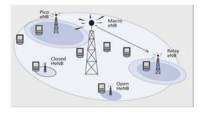
Fig. 1: A HetNet consisting of high powered and low powered cells [4]
