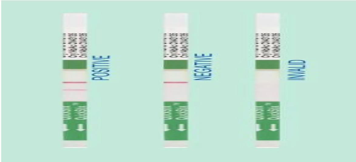
Figure 1: *Cry1Ab/1Ac Bt* strips showing positive, negative and invalid result (Envirologix, 2008)
