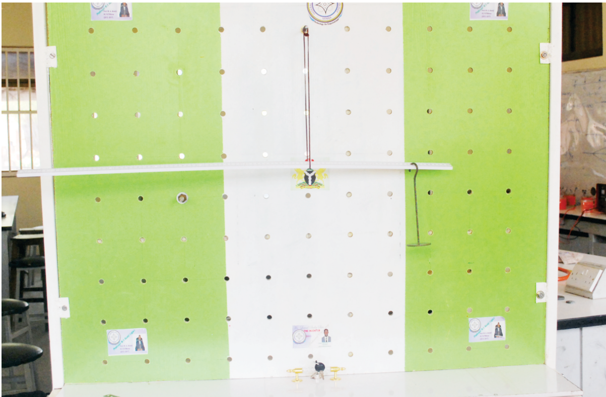
Fig. 13: Principle of Moment Experimental Setup
