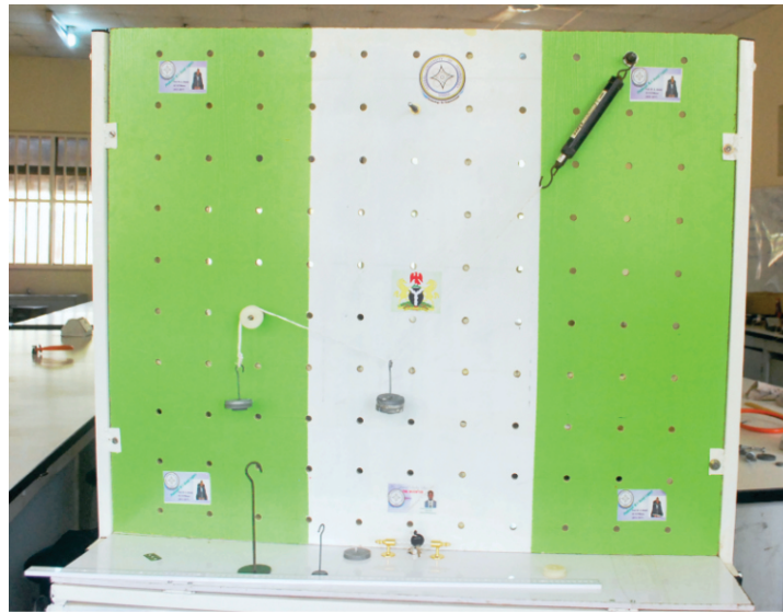
Fig. 14: Triangle of Forces Principles Experimental Setup
