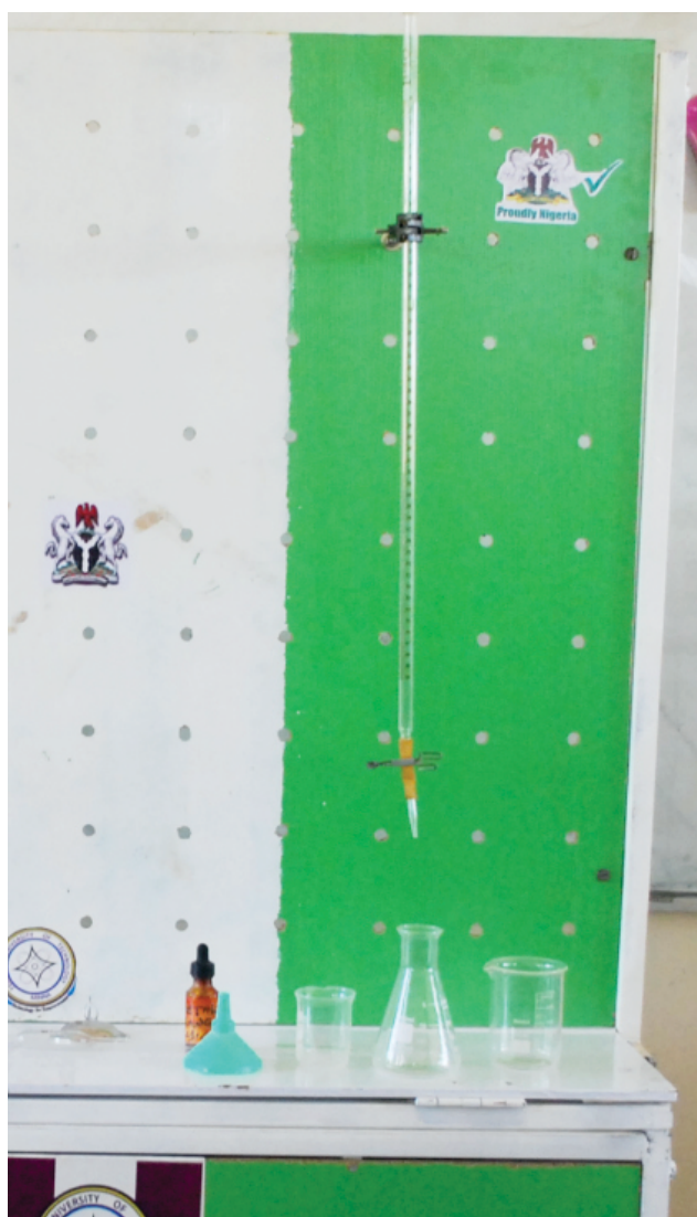
Fig. 16: Experimental Setup for Titration on the Mobile Laboratory
