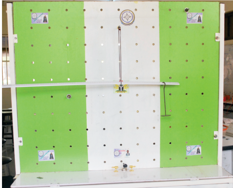
Fig. 8 : Moment Principle with Meter Rule
