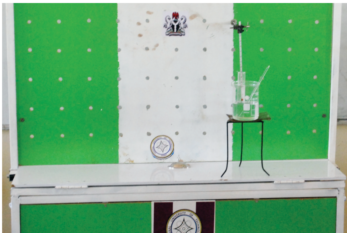
Fig. 20: Experimental Setup for Determination of Purity (Boiling/Melting Point) on the Mobile Laboratory
