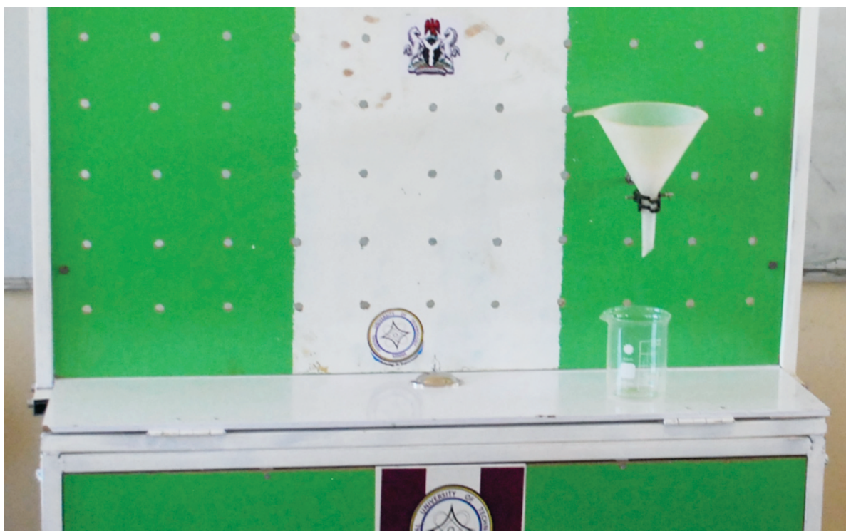
Fig. 19: Experimental Setup for Filtration on the Mobile Laboratory
