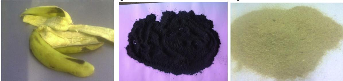
Figure 8a: **Banana Peel**      **Figure 8b:** carbonized (BCp)      **Figure 8c:** un-carbonized (BUNCp)
