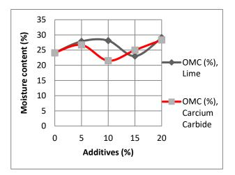
Figure 4: Moisture content of soil stabilized with for 0% - 20% Lime and Calcium Carbide
