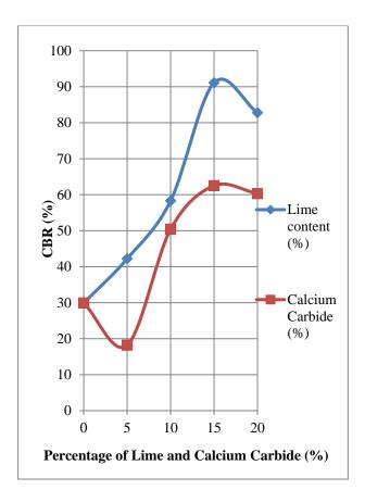
Figure 9: CBR of soil stabilized with Lime and Calcium Carbide residue
