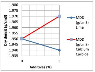
Figure 6: Dry density of soil stabilized with 0% - 5% Lime and Calcium Carbide additives
