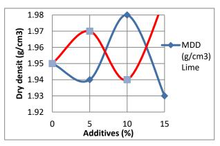
Figure 7: Dry density of soil stabilized with 0% - 10% Lime and calcium carbide
