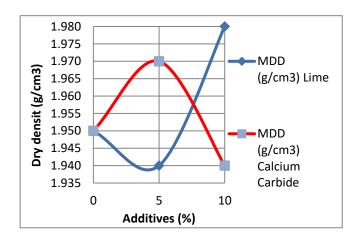
Figure 8: Dry density of soil stabilized with 0% - 15% Lime and Calcium Carbide
