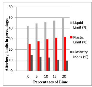
Figure 2: Atterberg Limit test for 0 - 20% Lime
