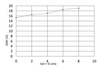
Figure 12: Variation of OMC of stabilized samples
