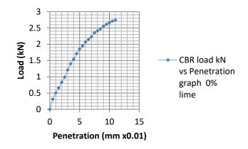
Figure 6: Load-penetration curve for natural soil
