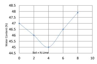
Figure 9: Variation of Liquid Limit with Soil + % lime
