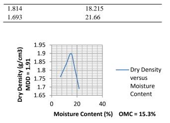
Figure 5: compaction curve for the natural soil at 0% lime
