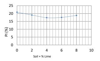
Figure 10: Variation of plasticity index of soil + % lime
