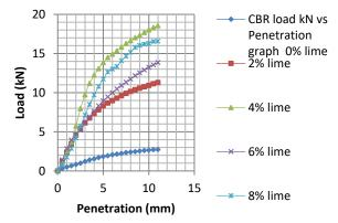
Figure 14: Load - penetration curves for stabilized soil
