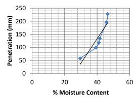
Figure 4: Penetration against moisture content
