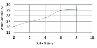
Figure 8: Variation of plastic limit with soil + % lime
