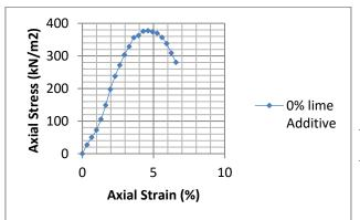
Figure 7: Axial stress – Axial strain curve for the natural soil
