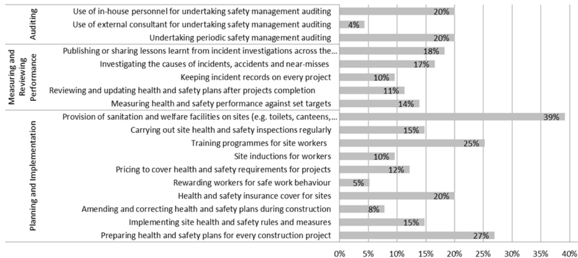
Figure 1: Level of Implementation of H&S Management Practices within Policy, Organising, and Risk Assessment
