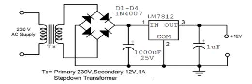
Figure 1.32: Schematic Diagram of a Regulated Power Supply System
