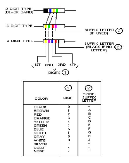
Figure 1.30: Semi-Conductors Coding System
