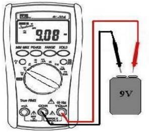
Figure 2.2: Test Leads Connected Across Component
