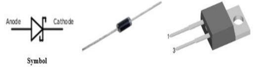
Figure 1.13: Circuit Symbol and Packaged Schottky Diodes
