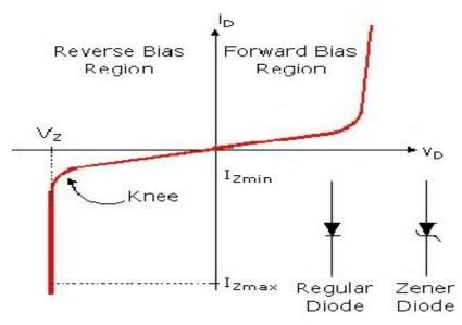
Figure 1.14: I-V Characteristics Curve of Zener and Regular Diodes
