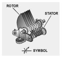
Figure 1.7: Shape and Circuit Symbol of Trimmer Capacitors
