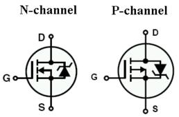
Figure 1.25: Circuit Symbol of a MOSFET
