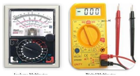
Figure 2.1: Analogue and Digital Multimeters
