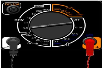
**Figure 2.4: Selector Switch Position**
