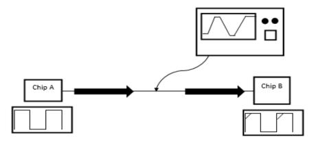
Figure 2.13: Real Probe Having Impact on Measured Signal
