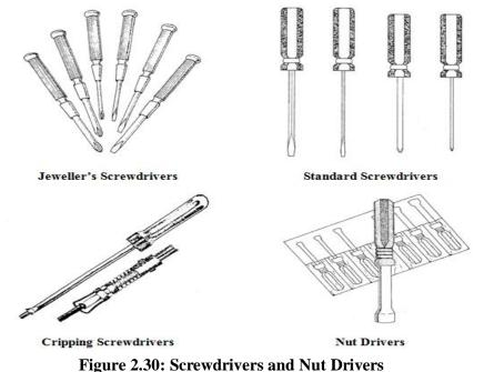
Nut drivers are like wrench sockets mounted to screwdriver handles. Like regular sockets, the socket-ends of the nut driver come in a variety of sizes and may be either standard or metric.
