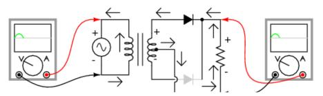
Figure 1.12: Full-Wave Rectifier with a Centre-Tap Circuit
