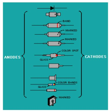
Figure 1.29: Polarities of Different Types of Diodes
