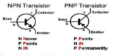
Figure 1.20: NPN and PNP Bipolar Junction Transistors
