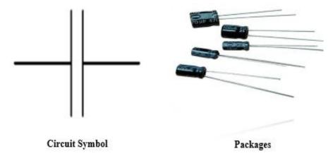
Figure 1.4: Circuit Symbol and Various Packages of Electrolytic Capacitors
