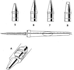
Figure 2.34: Interchangeable Soldering Iron Tips
