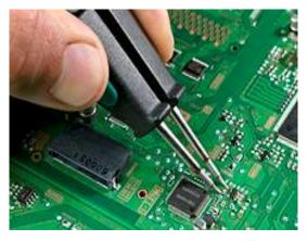
Figure 2.38: SolderingTweezers
