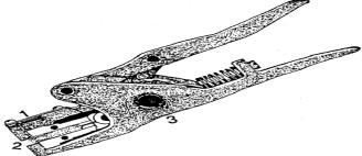
Figure 2.28: Automatic Wire Stripper
