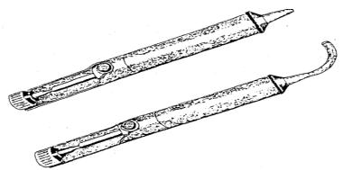
Figure 2.41: Unsoldering/Suction Pump
