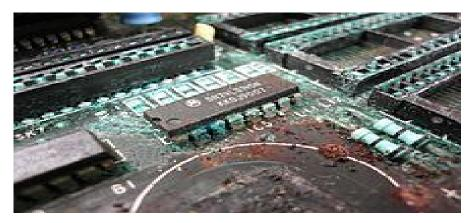
Figure 3.1: PCBCorrosion due to a LeakyMounted Battery
