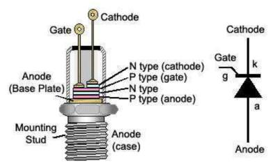
Figure 1.26: Cross-sectional View and Circuit Symbol of a Typical Thyristors
