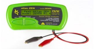
Figure 2.9: Model Atlas ZEN50 Zener Diode Analyser Source: Peak Electronic Design Limited (2015)
