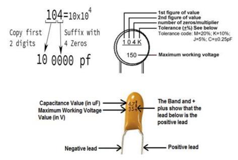
Figure 1.8: Methods of Evaluating Capacitive Values
