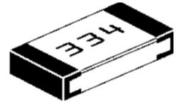
Figure 1.3: Surface-Mount-Resistor
