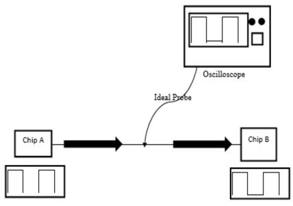
Figure 2.12: Ideal Probe Having no Impact on Measured Signal
