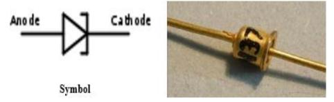
Figure 1.16: Circuit Symbol and Packaged Tunnel Diode
