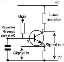
Ground (& Base) is Common to Input & Output Figure 1.23: Common Base Arrangement
