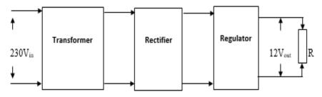
Figure 1.31: Bock Diagram of a Regulated Power Supply
