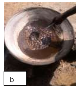
Plate II: (b) Formation of potash (MSAP)
