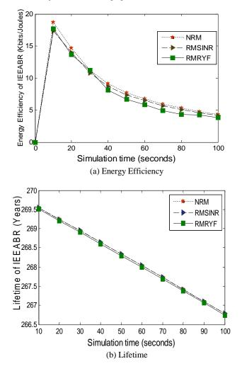
Figure 5: Energy efficiency and Lifetime comparison of IEEABR routing algorithm for different radio models (NRM, RMSINR and RMRYF).
