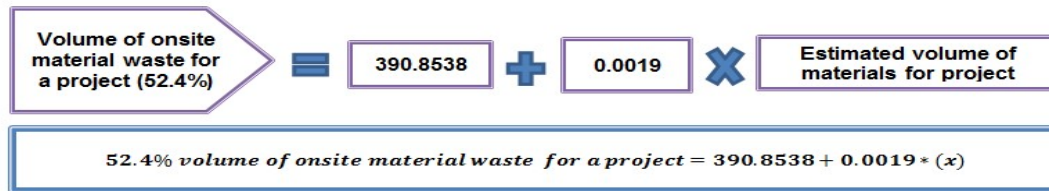
Figure 5: Mathematical model for predicting the volume of on-site material waste for a proposed project (52.4% completion)
