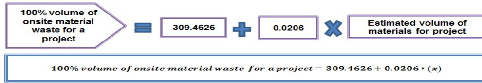
Figure 6: Mathematical model for predicting 100% volume of on-site material waste for a proposed project
