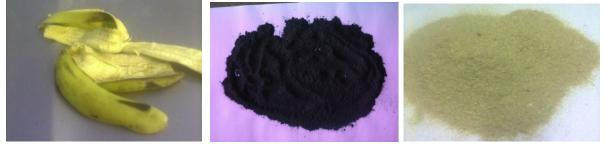
Figure 8a: **Banana Peel** Figure 8b: carbonized (BCp) Figure 8c:un-carbonized (BUNCp) (Source: Idris *et al.*,[5]).
