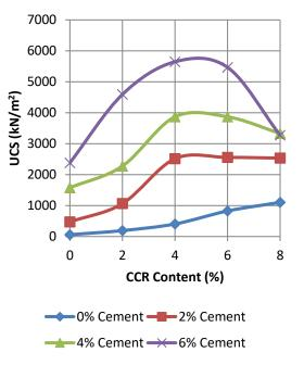
Figure 6: Variation of unconfined compressive strength with various dosages of cement and CCR after 28 days curing period
