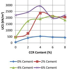
Figure 4: Variation of unconfined compressive strength with various dosages of cement and CCR after 7 days curing period
