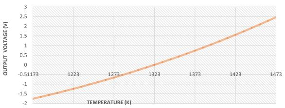
The Pyrometer Calibration Response
