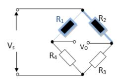
Fig 2 Bridge circuit of a bolometer (sensor)
