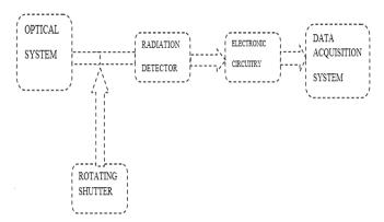
Fig 1 The block representation of the designed broad band chopped pyrometer
