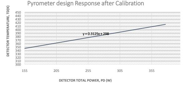
Fig 7 The Graph of Detector Temperature (K) against the Detector Total Power (W)
