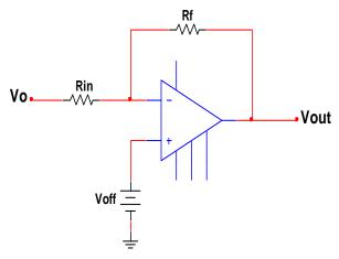
Fig 3 Diagram of an inverting amplifier for signal conditioning
