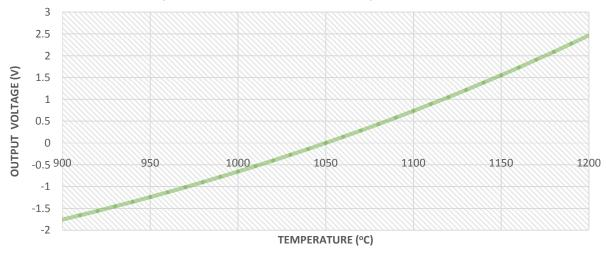
Fig 5 The Calibration Graph of Broadband Radiation Pyrometer Output Voltage (v) against Temperature (°C)
