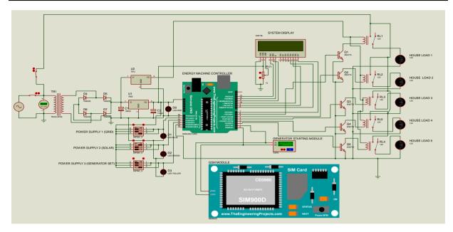
Figure 2: Proposed Mini-estate Intelligent Energy Machine Controller with Other Collaborative Supply Model
