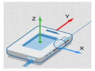
Fig 2: A Typical Accelerometer 3 D-Axis
