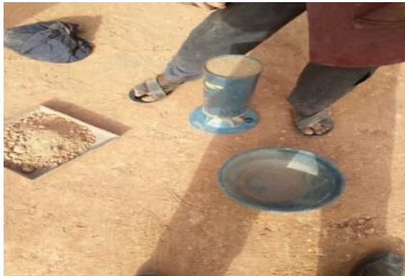
Figure 9: In-situ density test using the method of sand replacement
