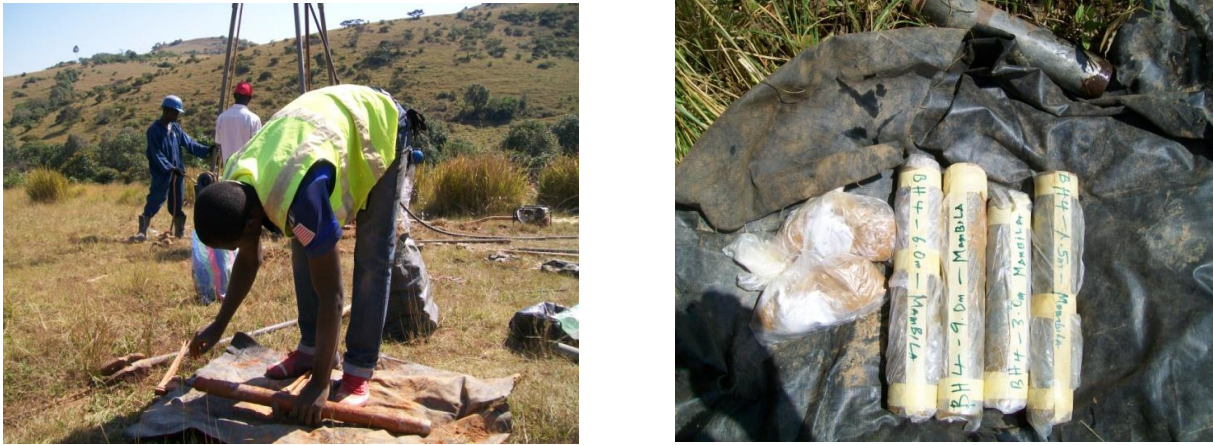
Fig. 2: SPT boring and sample collection in progress
