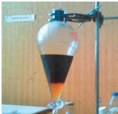
Plate III: Biodiesel in separating funnel
