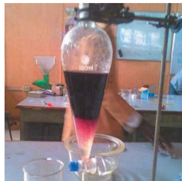
Plate II: Esterified oil in separating funnel
