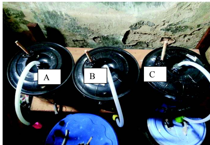
Plate 2: Experimental Set-up for Biogas Production
