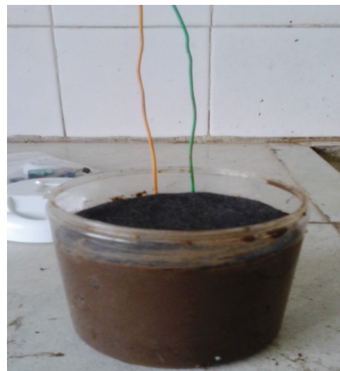
Figure 2: Anode and Cathode in MFC Vessel
